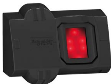
USB biometric switch dedicated to Schneider HMI (XB5S5)
