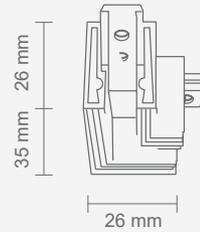
**CONECTOR CODO (INTERNO) AC5511N / AC5547N**
