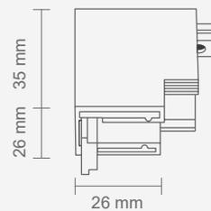
**CONECTOR CODO (EXTERNO) AC5512N / AC5548N**
