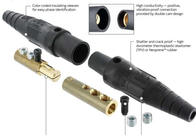
Self compensating for wear slit and in male contact provides spring action for longer usage Hard thermoplastic screw provides strength and durability
