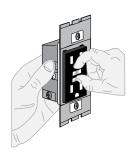
Pull out Test and Reset buttons
