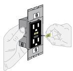
Insert new Test and Reset buttons
